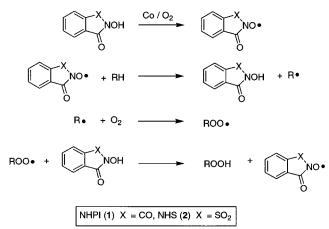
converted into its corresponding phthalimide *N*-oxyl (PINO) radical which is able to abstract a hydrogen atom from the organic substrate, thus propagating the autoxidation chain. In this way PINO is the actual chain carrier, which leads to longer propagation chains and, hence, to higher rates and selectivities compared to those from standard autoxidation.
